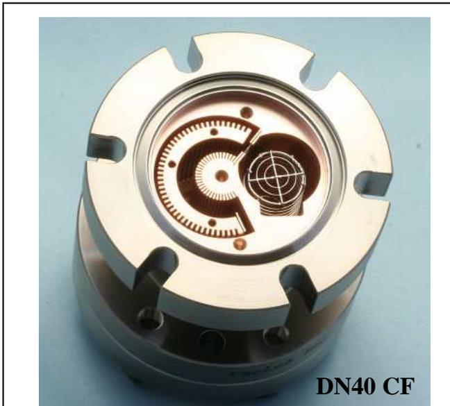
Top view of the 3BG-03, without the cover on the deflector and collector. The flanged mounting surface of the deflector can be seen in the picture, with its 3 mounting holes. Within the functional volume of the gauge, the deflector is an open array of bars and slots.
